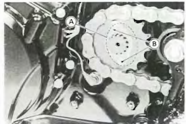
A. Sprocket Shoulder B. Engine Sprocket Bolts: Tighten to 9.8 N·m (1.0 kg·m, 87 in·lb)
